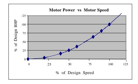
© Example: If the speed (rpm) of a 50 hp motor driving a pump or fan can be reduced from 1800 rpm to 900 rpm (50 percent), and still provide the necessary flow and pressure for the task at hand, the horsepower required is reduced from 50 hp to 13 hp resulting in a power reduction of 75 percent.
