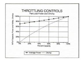
☺ The "Throttling Controls" graph above indicates that the compressor can operate continuously at any point between 0 percent and 100 percent capacity.
