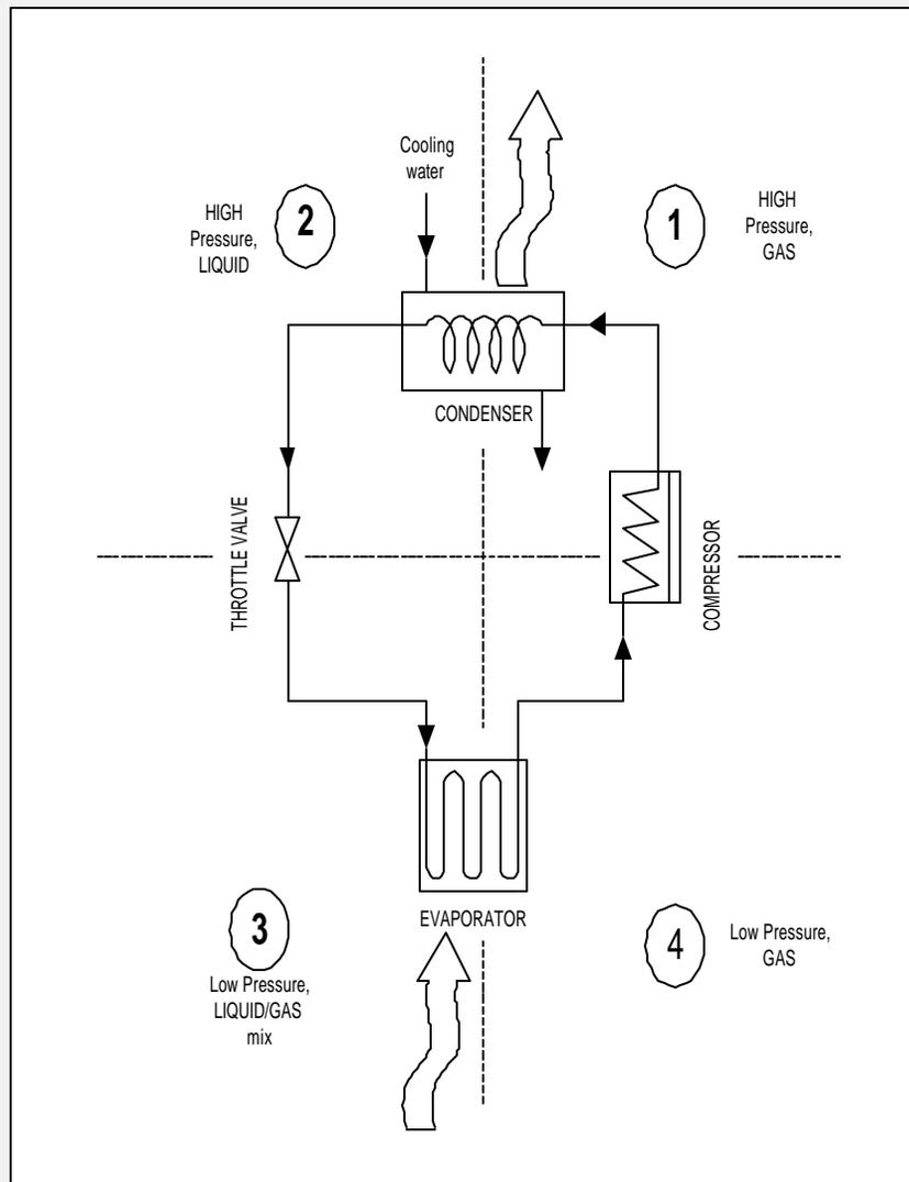
*Note: The “Simple Refrigeration Cycle” diagram is for information only and will be described in detail at a later time.*
