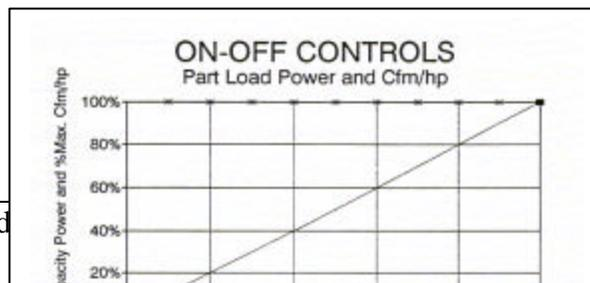
**Applications:** This type of control strategy works best when the user is confident that there will be long periods of either very high or very low use, and when the maximum and minimum pressures are not close together. Large receivers are required for efficient operation. A small plant with an occasionally used sandblaster would be an appropriate application for this control strategy.
