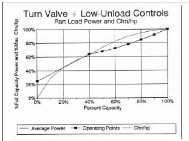
⊗ Note: Since spiral/turn/poppet valves are already efficient in the higher capacity region, available savings from increasing the unloading point are less significant for compressors with this type of control. This can be seen by referring to the “Turn Valve + Low-Unload Controls” graph above, if the unloading point is moved from 40 percent to 80 percent, the area under the curve is not significantly reduced.
