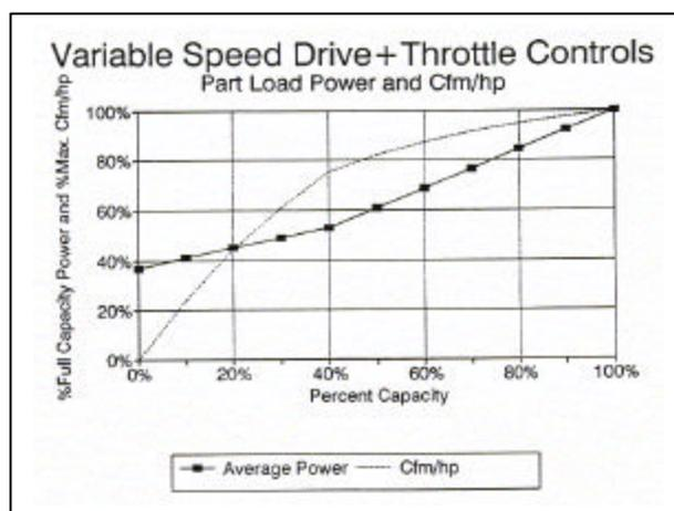
*Note: VSD + Throttle Controls graph shows VSD control down 40% capacity and Throttle Control down zero to 40% capacity.*
